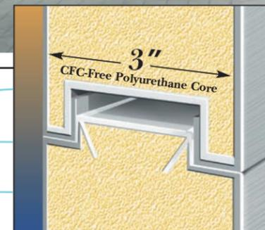
With a solid 3" core of high-density polyurethane foam insulation, Haas Door's ThermaPro™ sectional steel door meets the most demanding specifications, while providing a calculated R-Value of 25.8.
